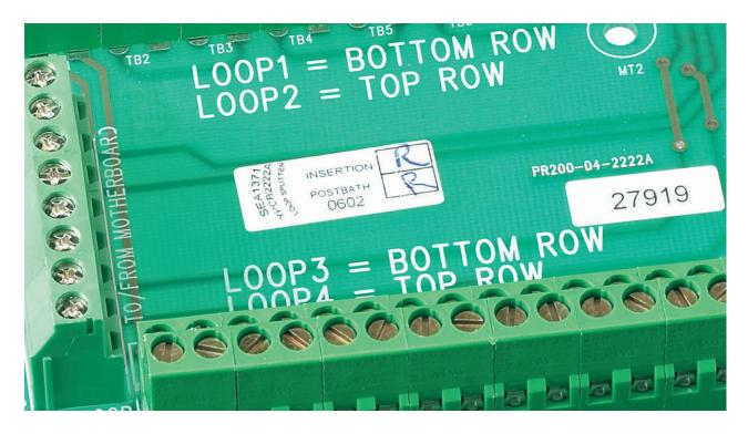
The loop splitter interface (ZPCB2222) allows the expansion of the Eaton CF3000 from a 4 loop panel to a 16 loop panel.
