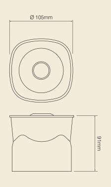
The Symphoni AV provides a solution to the increasing need to incorporate visual alarms as well as sounders into fire systems. The compact combination of LED beacon and Symphoni style sounder is extremely efficient making it ideal for system extensions and upgrades without adding undue loading to power supplies or sounder circuits.
